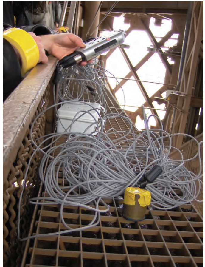
Fig. 8. Geophone positioned on the metal grating in the service stairwell underneath the summit. Credit: France Languérand.
