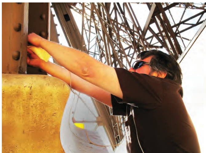
Fig. 4. Seth Horowitz placing the seismic sensor on the iron at the base of the Eiffel Tower. Credit: China Blue.
